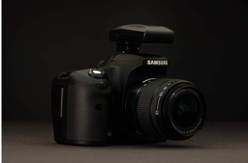
Geotagging photos is as simple as releasing the camera's shutter with Geotate's Kato accessory design. Just attach the device to the camera's external flash hot-shoe connector and each time a photo is taken the location is captured instantly and automatically. The design can be brought to market rapidly and at low risk through an OEM model provided by Goobie.
